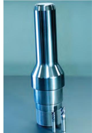
*Fraunhofer coated 15" long spindle punch for high temperature forming process (end mills in front are for size reference)*
