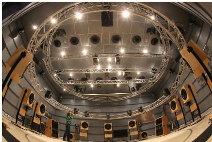
*HE-AAC and other audio codecs are developed and tested in Fraunhofer's advanced sound lab that allows for critical listening and flexible loud speaker arrangement.*
